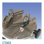
Adjustable jaws Rubber-edged arms may be independently repositioned to accommodate unique samples.
