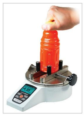
Series TT01 Cap Torque Testers are designed to measure application and removal torque of bottle caps up to 100 lbFin [11.5 Nm]. Adjustable posts effectively grip a broad range of container shapes and sizes, while optional flat and adjustable jaws are available for unique profiles. A rugged aluminum design, and simple, intuitive operation allow for use in laboratory and production environments.
